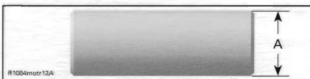
A. Piston pin diameter in the area of the bushing.
